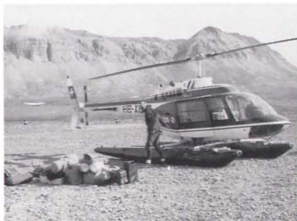
Fig. 10. Bell 206 Jet Ranger helicopter with equipment for a two-man geological field camp being loaded.
