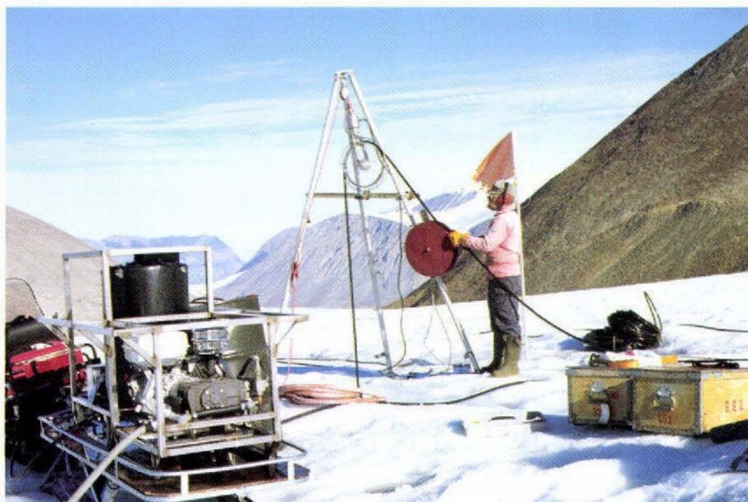
Fig. 3. Hot water drilling for installing thermistor string at stake 451 on Hans Tausen Iskappe.
