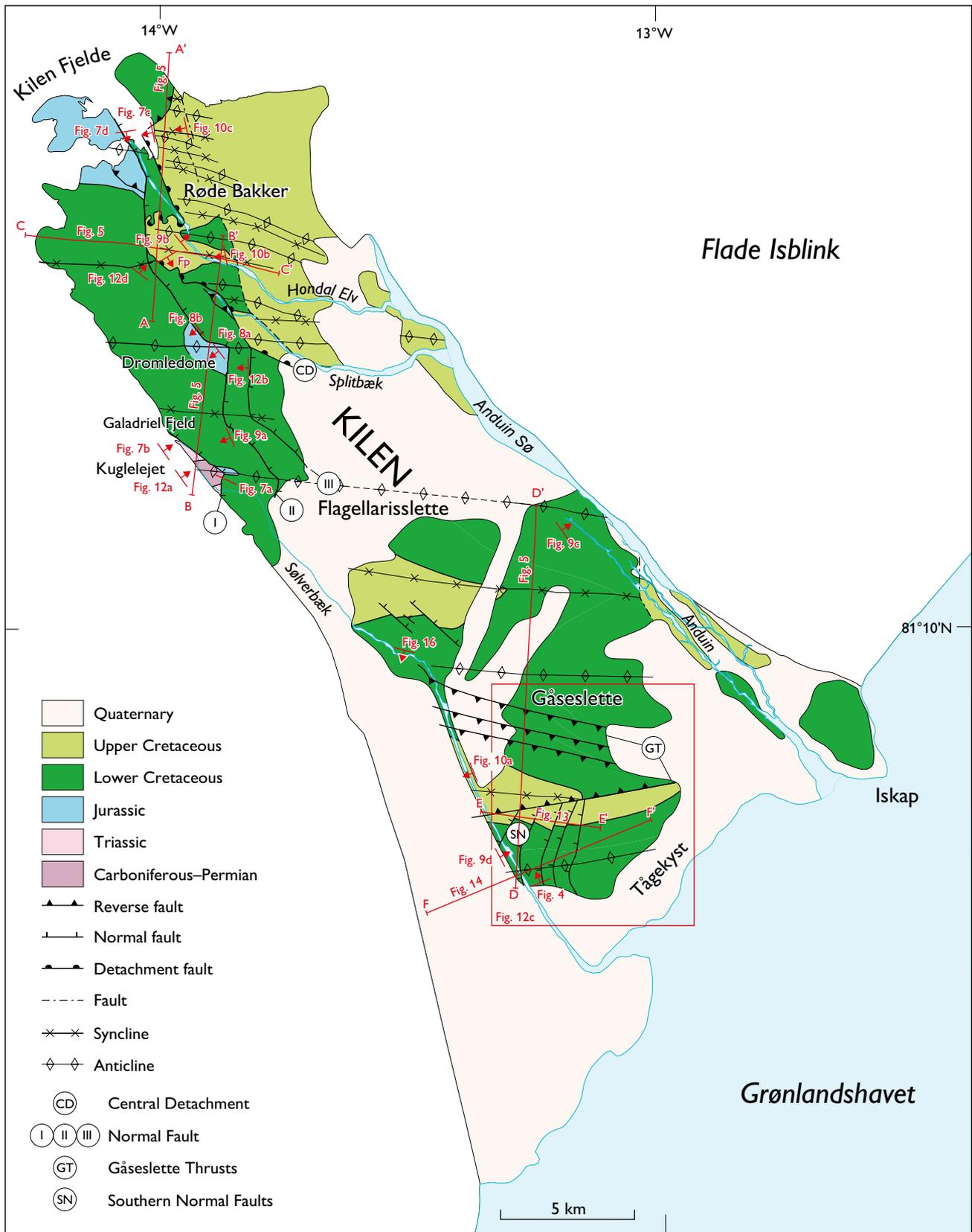
Fig. 2. Simplified geological map of Kilen. The Galadriel Fjeld Formation is included in the Lower Cretaceous, although it includes strata belonging to the lowermost Upper Cretaceous. The positions and direction of view of images on the frontispiece (Fp) and in Figs 4, 7–10, 12 and 16 along with cross-sections in Figs 5, 13 and 14 are shown. Modified from Svennevig *et al.* (2016).
