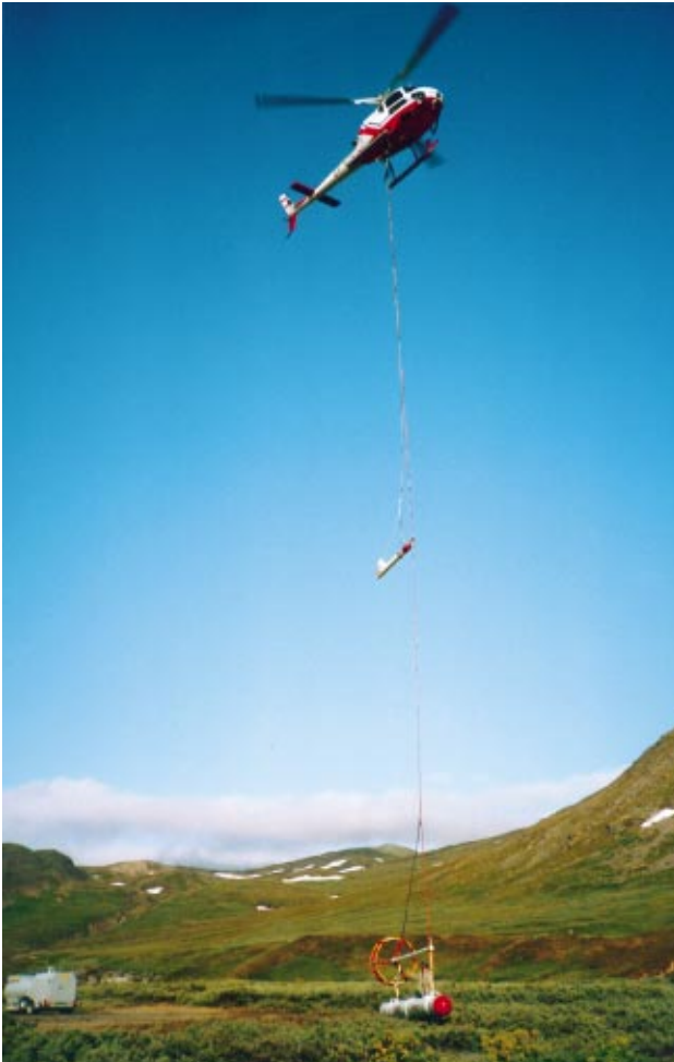
Fig. 3. The Greenlandair helicopter taking off from Grønnedal with the Aerodat bird assembly. Magnetometer and VLF sensor in midair, with electromagnetic transmitter/receiver system on ground.
