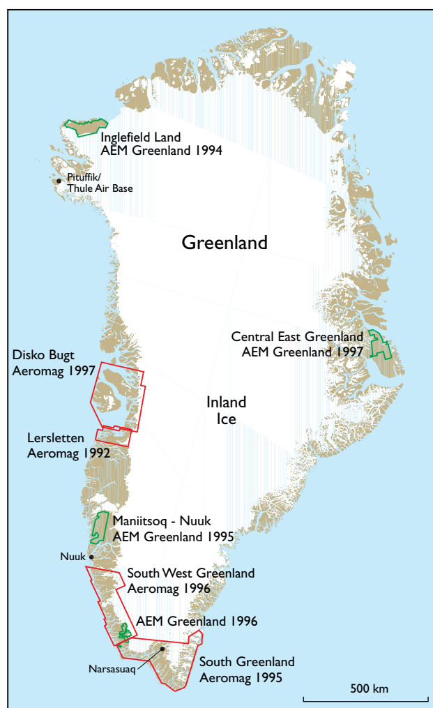
Fig. 1. Airborne geophysical surveys in Greenland 1992–1997. Project AEM Greenland surveys outlined in green, Project Aeromag in red.
