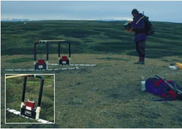
Fig. 4. The pulse EKKO IV georadar system in use at site 638 (see Fig. 3 for location). GPR is in reflection mode. The GPR consol, portable computer and power source are carried by the geologist and linked with fiber optic cables to two 50 MHz antennas.
