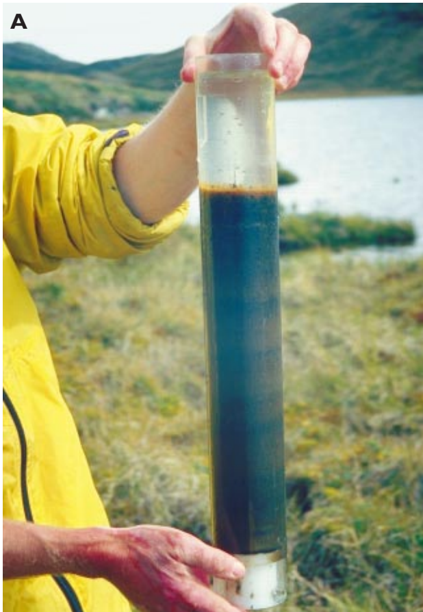
Fig. 4. A: Typical Kajak core with unlaminated sediments from a freshwater lake. B: Extruding a Kajak core in the field.
