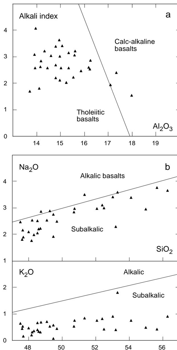
Fig. 18. (a) Alkali index *v.*  $Al_2O_3$  (after Middlemost, 1975). (b) Variation diagrams of  $Na_2O$  and  $K_2O$  *v.*  $SiO_2$  of homogeneous amphibolite, Fiskefjord area, illustrating its tholeiitic character. Locations of samples in Fig. 17; analytical details in Appendix.
