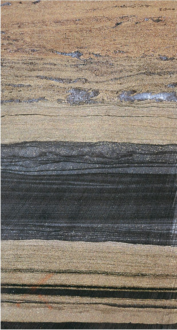
Fig. 16. Fine-grained laminated sulphides in black mudstone. The sulphide laminae consist of framboidal pyrite in a matrix of sphalerite and carbonate. Zn-content in the upper sulphide layer is 25–30% and in the lower layer 1–3%. Platinova drill-core CF-15 in Level 2 mineralization; figured in Kragh (1996). The core is 3.6 cm across. Photo: Jakob Lautrup.
