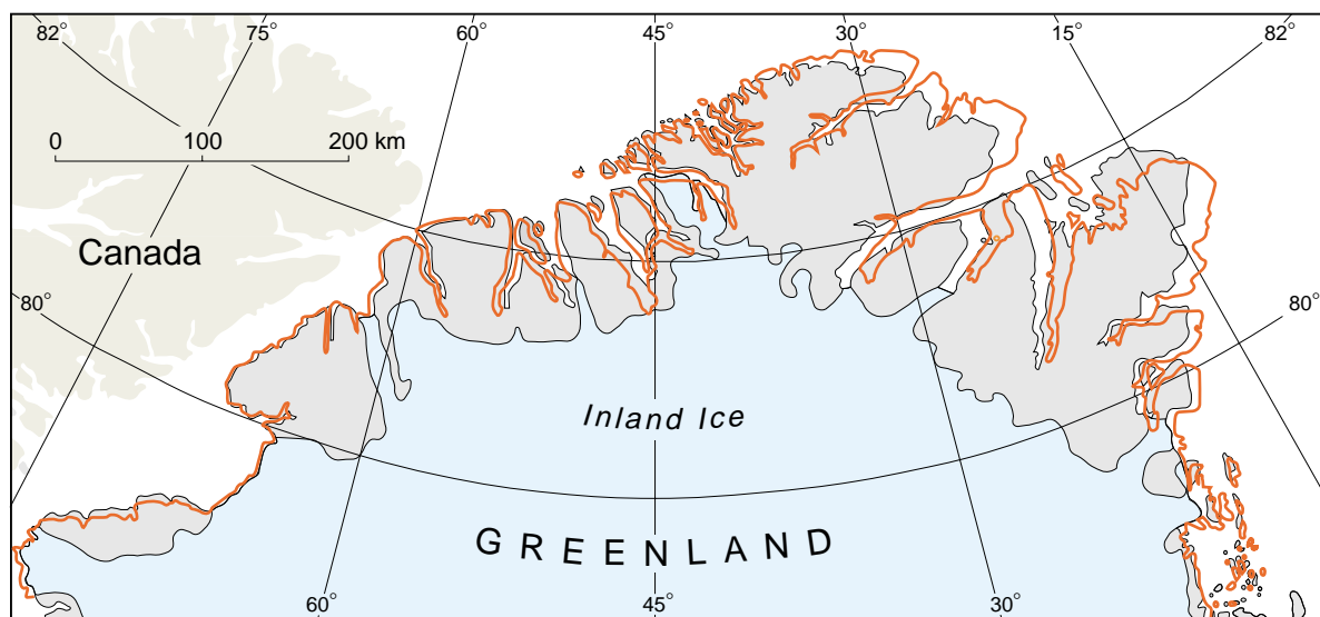
Fig. 2. Outline map of North Greenland showing misplacement of boundaries between land and sea on respectively old (black) and new (red) topographic maps. The new map outline in red is based on ground control points measured in 1978. Data from Kort & Matrikelstyrelsen, Copenhagen, Denmark.
