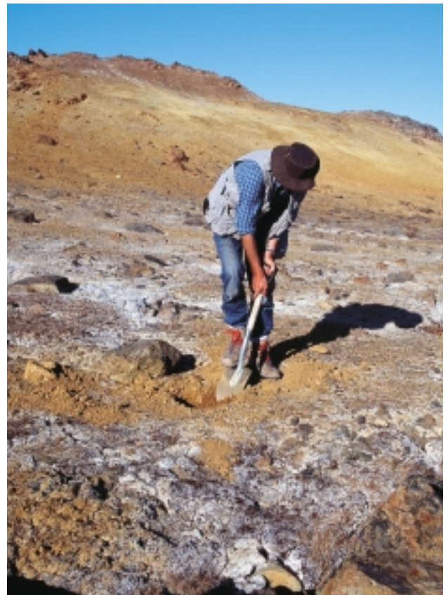
Fig. 9. Geochemical sampling of soliflucted material from a rust zone in paragneisses, 10 km south of Marshall Bugt, central Inglefield Land. Analysis of the soil samples here gave up to 75 ppb Au, 101 ppm As, 172 ppm Cu and 235 ppm Zn.
