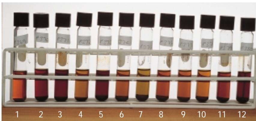
Fig. 4. Pigment extracts from consecutive samples down a freeze core from Brayasø: left to right, from surface to about 7 cm depth. The darker red coloration visible in samples 2, 3, 5 and 12 is caused by a pigment (Okenone) produced by purple-sulphur bacteria that can be seen as purple bands in the original sediment.
