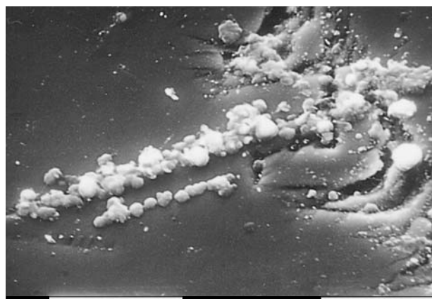
Fig. 3. Secondary \text{Cu}_2\text{S} growth along polishing scratches and contorted cleavage on the surface of polished thalcosite. Compare with Fig. 1, top centre SEM image. Scale division 10 \mu\text{m} . Sample GM 2001.1 (Geological Museum, Copenhagen).
