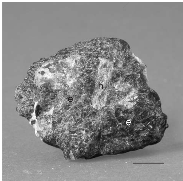
Fig. 2. Hand specimen (sample 104378, Geological Institute, University of Copenhagen) showing crystal of hiortdahlite ( h ) enclosed in eudialyte ( e ), scale = 1 cm. Photo: Ole Bang Berthelsen.
