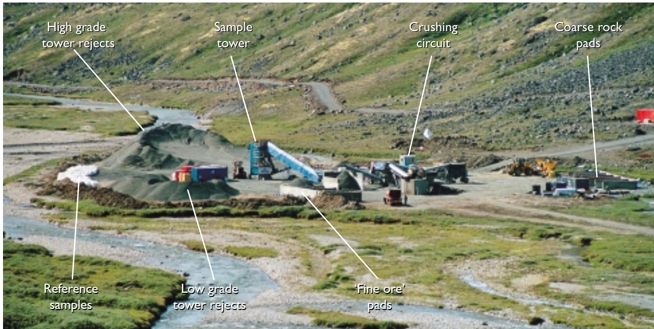
Fig. 6. Crushing and sampling plant at the valley floor below the 'Nalunaq' mountain (c. 500 m south of the camp in Fig. 2). See text for description of sample flow. Note the front-end-loader beside the sample tower and the person near centre of photograph for scale. Photo: Hans Christian Langager.
