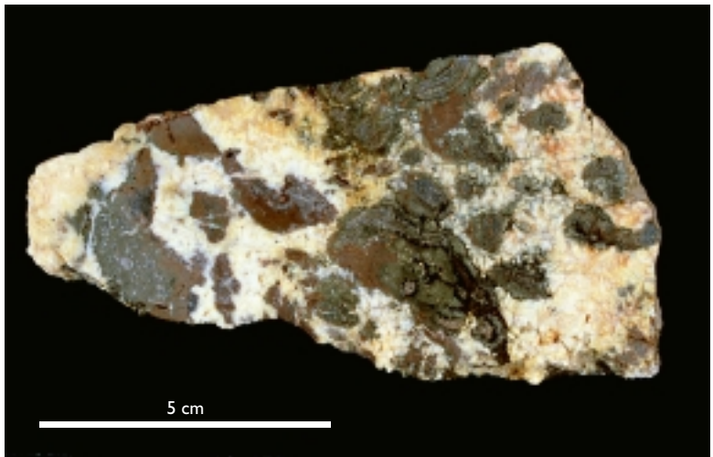
Fig. 4. New Zn-Pb-Ag occurrence, eastern Washington Land: cut slab of boulder sample. Coarse-grained dolomite with large sphalerite aggregates – note colloform-banded pyrite and sphalerite in central part of slab (sample GGU 447027: 15% Zn, 0.4% Pb).
