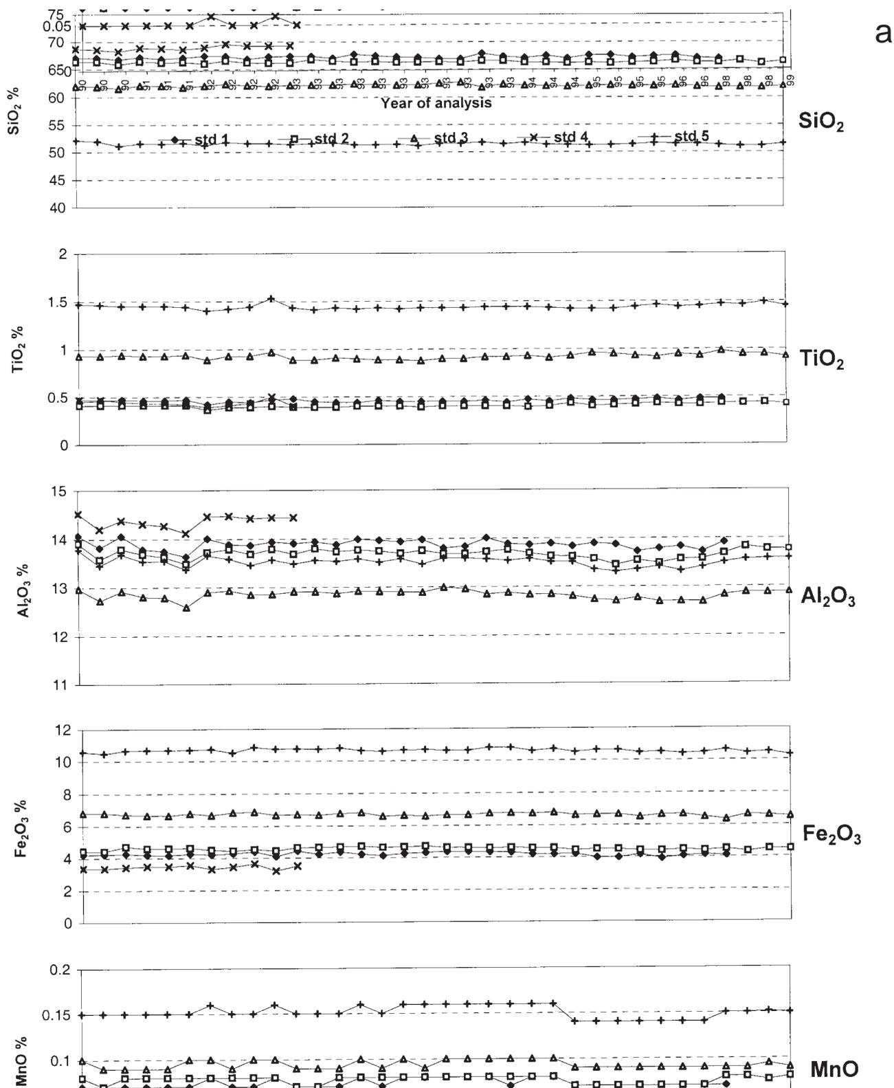
Fig. 1. **a, b:** Variability of major element results for five internal standards (std 1–5) in the period 1990 to 1999. The standards are analysed by simultaneous X-ray fluorescence spectrometry on glass discs and atomic absorption spectrometry (for Na) at the Rock Geochemical Laboratory, Geological Survey of Denmark and Greenland. Fe<sub>2</sub>O<sub>3</sub> is total iron.
