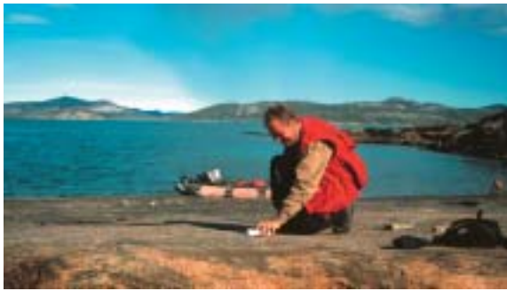
Fig. 2. The hand-held magnetic susceptibility meter is small and easy to use. Measurements are taken first with the meter at the rock surface, followed by a reference reading with the meter held up in the air. The photograph shows the first step of the measurements on typical gneiss lithologies in the central part of Ussuit fjord.
