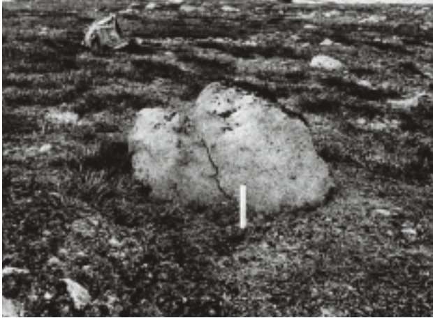
Fig. 6. Weathering of a tholeiitic diabase boulder at Site 22. The photograph of the rock in 1960 ( left ) was taken before a linen sheet was placed under the rock to collect weathering products for quantitative calculations on granular disintegration. White ruler is 17 cm long. The sheet had almost disintegrated by summer 2000 ( right ). It is evident from the two photographs taken 40 years apart that granular disintegration has been substantial in this arctic environment.
