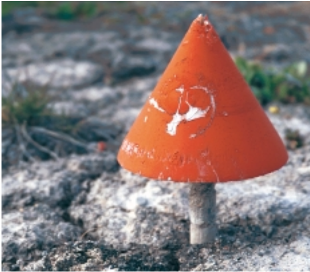
Fig. 2. Close-up of target cone in mass-wasting target line at Site 5 in the summer of 2000. The 10 cm high wooden cone mounted on a wooden peg was inserted into the ground in 1956.
