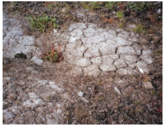
Fig. 4. Experimental Site 9 originally instrumented with short dowel sticks 0.3 cm in diameter. The dowels were spaced at intervals of 10 or 20 cm at the beginning of the experiment and inserted to depths of 5 or 10 cm in lines or grid patterns ( left ). The original dowel patterns established in the late 1950s were found to be obliterated when revisited in 2000 ( right ), due to up-freezing by the intervening freeze–thaw cycles. Arrow indicates one of the uprooted dowel sticks.
