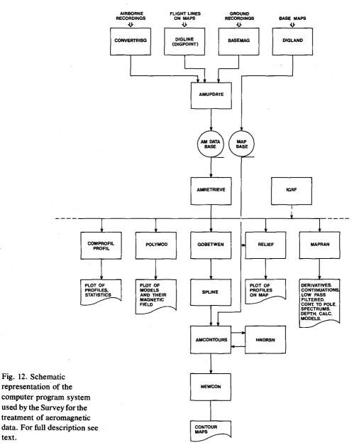
outputs (Tektronix screen or CalComp plotter) as well as the results used in further processing. The AM system is continuously being updated and optimised, and new programs are being added.
